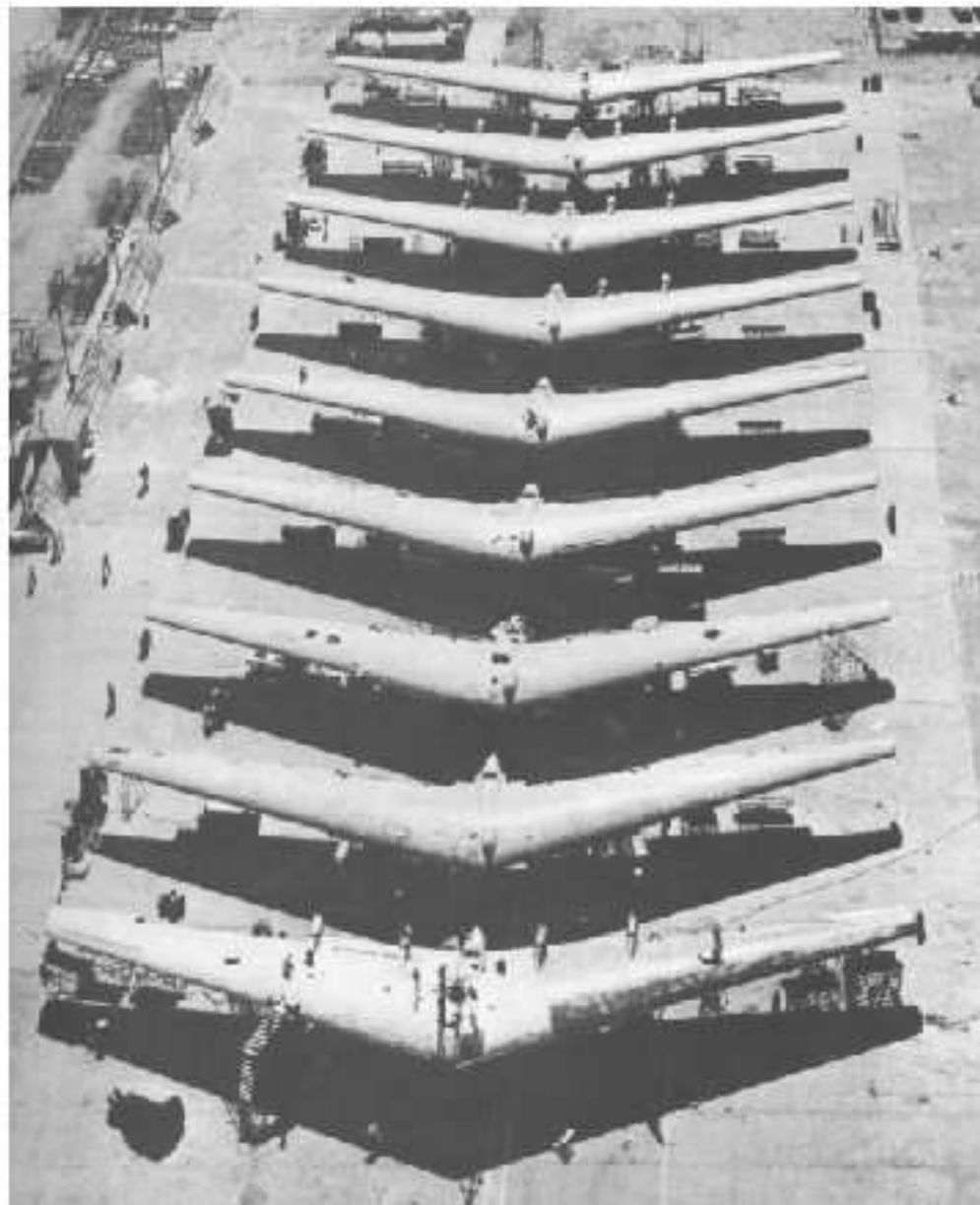
this is a rare photo of nine Northrop Flying Wing Bombers. Many people do not realize that more than one or two prototypes were built of this design. Here, for the first time, is actual proof of their existence. Two of the big wing bombers are undergoing modifications from XB-35's to Flying Wing B-49 1t Bombers. The entire project was later cancelled by the Air Force.
